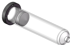
1.5 Put the rubber piston into the cartridge & The cartridge fixing seat is rotated and installed on the cartridge./ 将橡胶活塞放入料筒中，料筒固定座旋转安装在料筒上。
